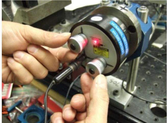
**Figure 23** – Use laser micrometers to trim out angular errors
