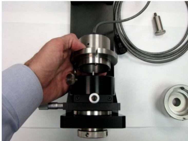
Inserting T-218 Target in X-Y Stage
