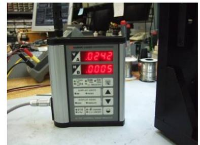
Figure 17 – R-1307 showing Vertical reading of +.0250 in.
