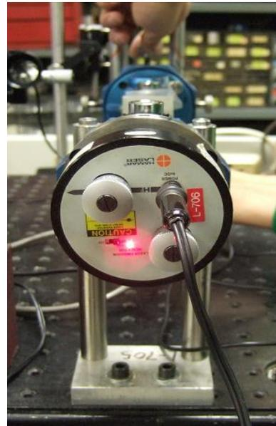
Figure 21 – Invert L-705 Laser 180 degrees
