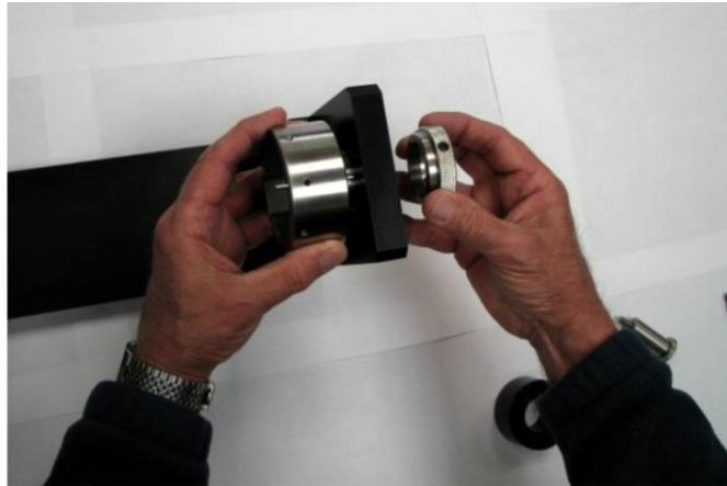
T-218 Target Centering Adapter Mounting
