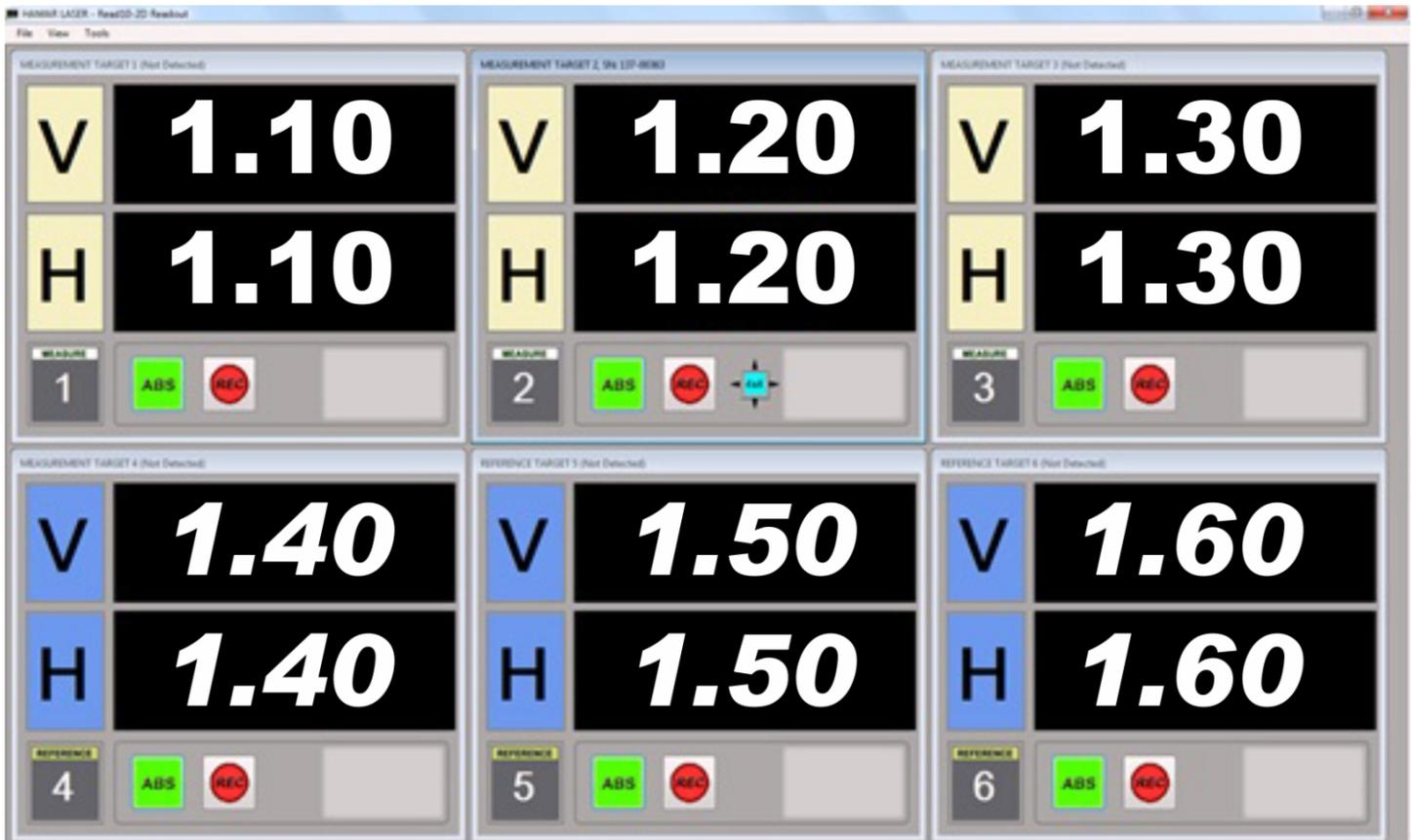
*The Read10-2D Readout Data screen can display readings from six targets (3 measuring targets and 3 reference targets). When using fewer than six targets, the data display screens expand in size, allowing a single target screen to be viewed from as far away as 50 feet.*
