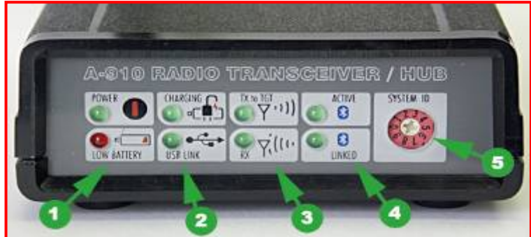
Figure 18 – The A-910 Radio Transceiver/Hub FRONT PANEL
