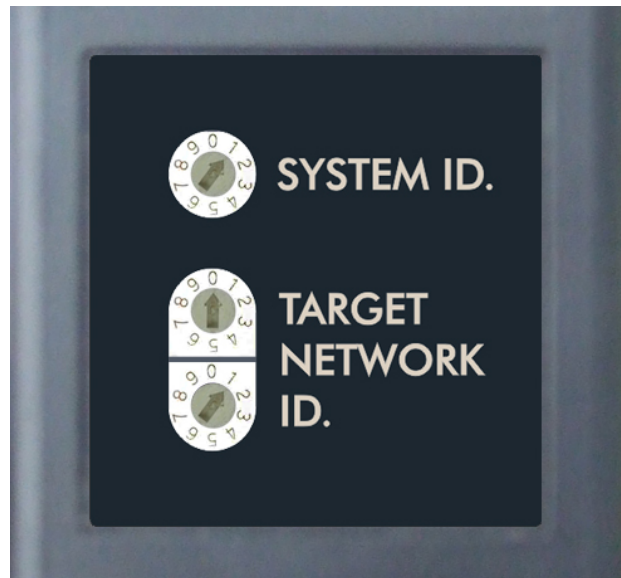
Figure 25 – Unitarget ID Switch set to 1
