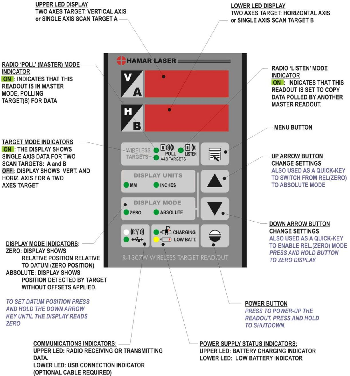
Figure 6 – R-1307W Readout Control Panel Features
