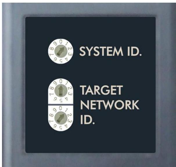
Figure 25 – Unitarget ID Switch set to 1
