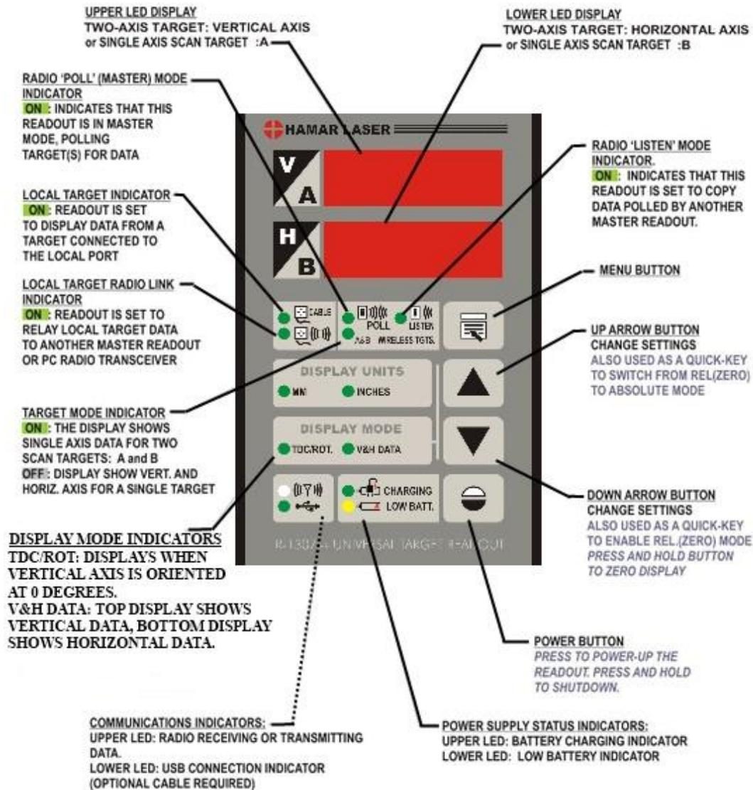
Figure 8 – R-1307+R Readout Control Panel Features
