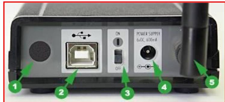
Figure 19 – The A-910 Radio Transceiver/Hub REAR PANEL
