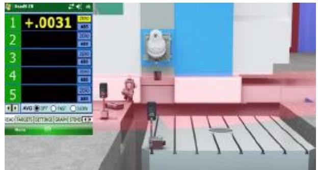
5. Plane5 analyzed the data and found that the flatness of rotation is .0010 in. TIR and the parallelism to X is .0011 in/ft and .002 in/ft to Z.
