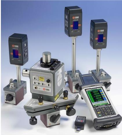
The L-733 Triple Scan Laser was specifically designed for machining centers to measure and correct machine geometry. It has all of the innovative and highly useful features of the L-743 Ultra-Precision Triple Scan Laser, with lower accuracy and a medium adjustment base. It is very useful for checking the alignment of large fabrications or aligning large airplane sections in aircraft manufacturing.
