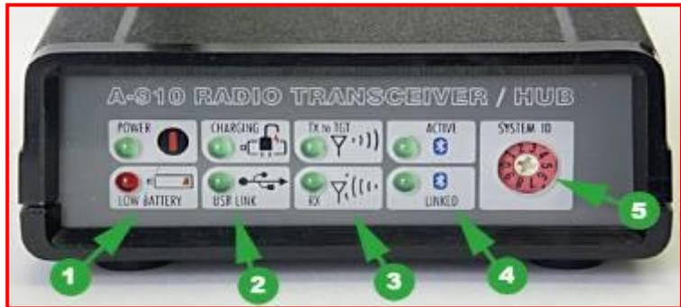
Figure 33 – The A-910 Radio Transceiver/Hub FRONT PANEL
