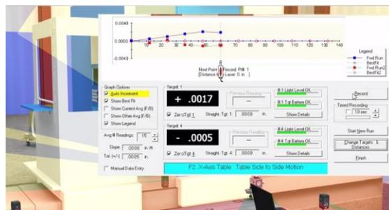
5. The X-Axis results show a Straightness error of .0007 in. TIR and a Flatness error of .0006 in. TIR. The slope of the Best Fit line is .0003 in/ft, which means the X-Axis is sloping UP relative to the table.
