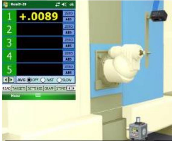
2. As with the A-axis, begin at 0 degrees, zero and rotate 180 degrees. The .0031 reading indicates the spindle axis is pointing upward relative to the Y-axis.
