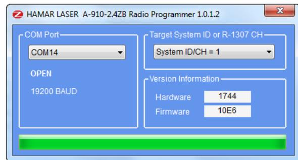
Figure 36 – A-910 Utility showing the COM Port, System ID and Channel settings
