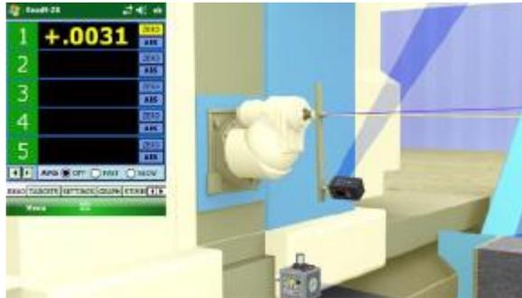
3. To compare the X-axis, start at 90 degrees and zero the PDA. Rotate to 270 degrees. The -.0019 reading indicates that the spindle axis is pointing to the left relative to the X-axis.
