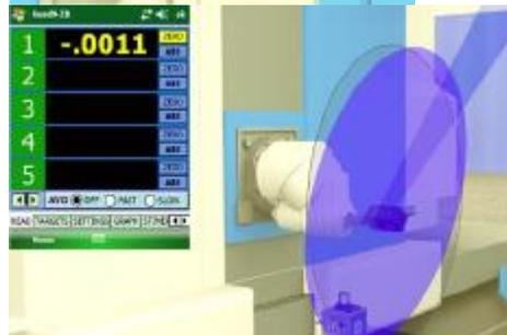
4. Rotate to 90 degrees and zero the target.
