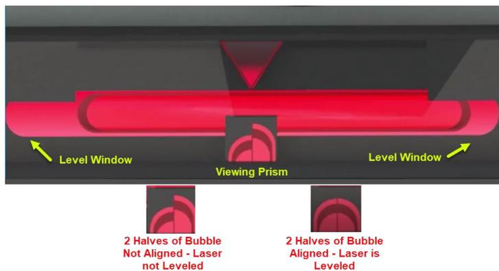
Figure 10 –L-740SP Split-Prism Level Vial Assembly for L-740 Series Lasers
