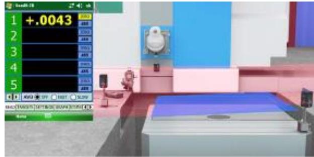
4. The last reading is .0031 and the data is uploaded to Plane 5 for analysis.
