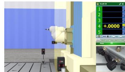
4. Return the column to its starting position and rotate the target toward the laser. Zero the target.
