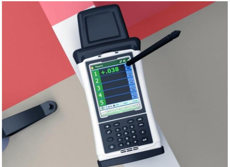
5. “Buck in” or tilt Laser Plane #1 (LP#1) using the Yaw Adjustment until Target #1 reads zero at the Far Point. Move Target #1 back to the Near Point, re-zero, and repeat the process until the target reads zero at both locations, which usually takes 2-3 tries. If using the Remote Buck-in Formula (see Page 64), this process can be done in one pass.
