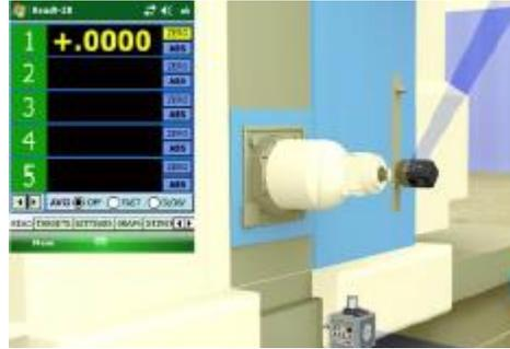
5. Rotate to 270 degrees. This reading is  $-.0023$ , which means the A rotation axis is tilting toward the X-axis by  $.0023$  in 18 in.
