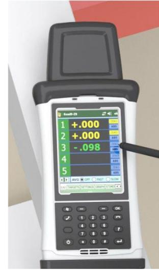
**Figure 22** -- R-1356-2.4ZB PDA Readout showing data values for Targets #1, 2 and 3
