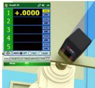
3. Rotate the A-axis 180 degrees. In this case, the reading is -.0011, which means the A rotation axis is tilting forward relative to the Y-axis by .0011 in 18 in.
