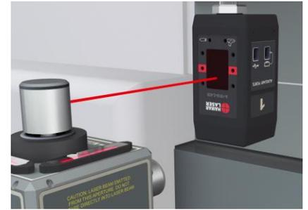
2. Turn on the rotation for both laser planes. The Gold Laser (top left) measures X-Axis Straightness and the Red Laser (bottom left) measures Flatness.
