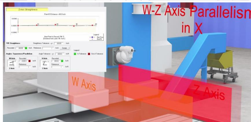
6. For Z squareness to X and Y, the Machine Tool Geometry program subtracts the Best-Fit slope of Z from the Best-Fit slopes of Y and X and calculates the squareness. Therefore, the result for the squareness of Z to X is .0002 in/ft, which means the Z-Axis is tilting to the left.
