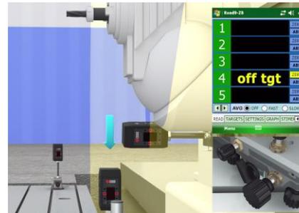
5. Send the column back to the far end of travel and tweak the Yaw-Axis adjustment knob to zero the laser.
