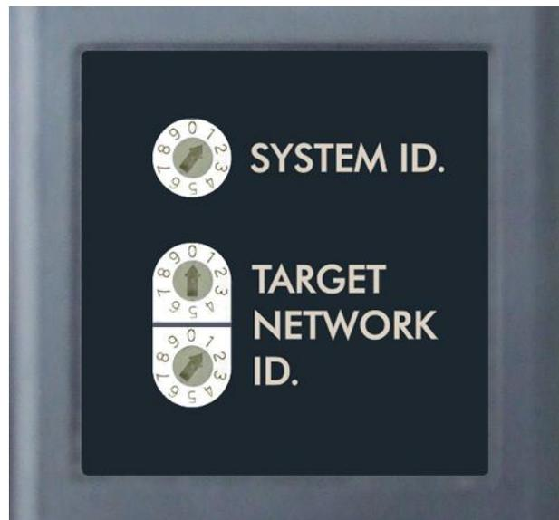
Figure 38 – Unitarget ID Switch set to 1
