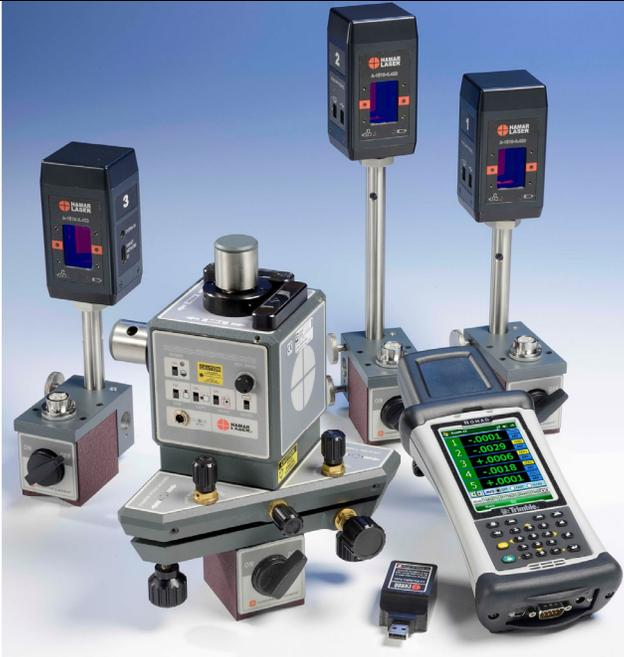
The L-743 Ultra-Precision Triple Scan® Laser is the ideal instrument to quickly and accurately calibrate the geometry of almost any kind of press. The critical alignment of any press is the parallelism of the upper and lower rams to each other and squareness to the way (gib). The ways also need to be parallel. Poor alignment results in poorly formed parts that need to be scrapped and excess wear and tear on the press itself.
