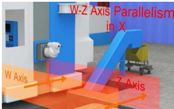
1. To set up for W, change the target position, turn on the laser rotation and adjust the spindle to center the laser.
