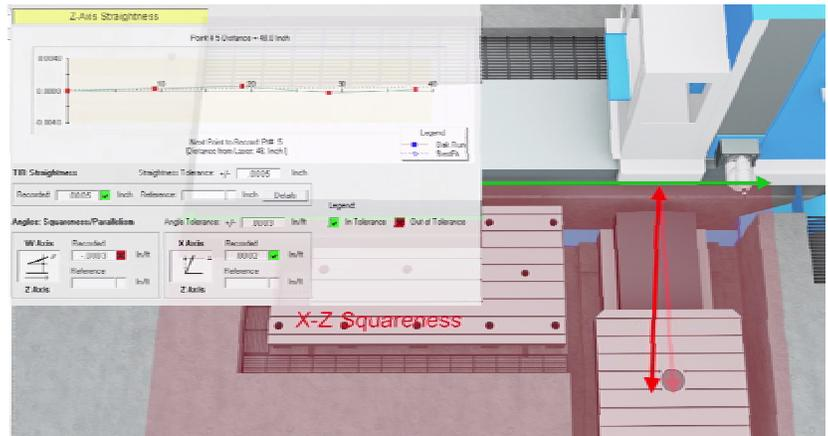
7. The squareness of Z to Y is .0004 in/ft, which means the Z-Axis is sloping up relative to Y.
