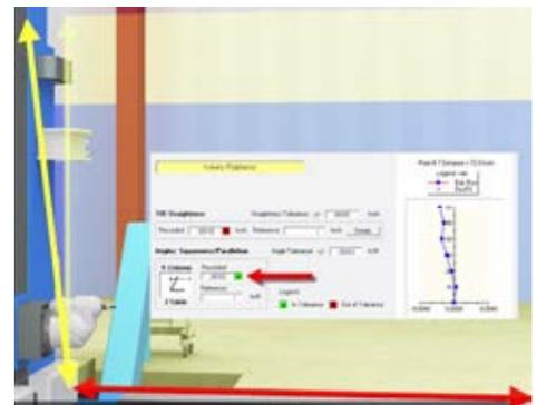
**W-Axis Flatness and Straightness, W-Z (in X) Parallelism, W-Z (in Y) Parallelism**
