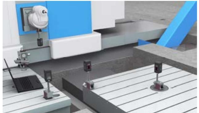
2. For straightness, mount Target #2's post into the side hole in the magnetic base to pick up the green laser plane. Adjust the pole length for Target #2, turn on the green laser and zero the display.
