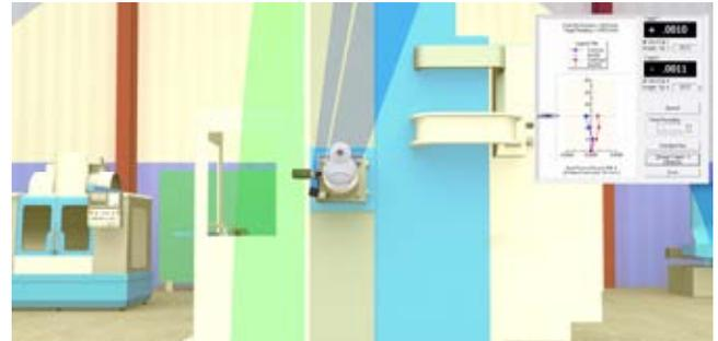
5. As before, the Machine Tool Geometry software does the straightness and squareness calculations. The results show .0010" TIR for flatness and .0008" TIR for straightness.
