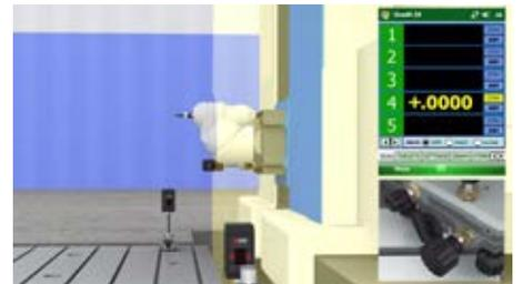
4. Return the column to its starting position and rotate the target toward the laser. Zero the target.
