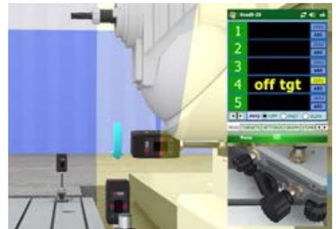
5. Send the column back to the far end of travel and tweak the Yaw-Axis adjustment knob to zero the laser.
