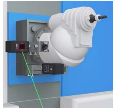
2. Turn on the laser rotation and zero the targets.
