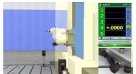
6. When the target reads zero at both ends, the laser is aligned to the X-Axis.
