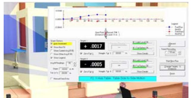
5. The X-Axis results show a Straightness error of .0007" TIR and a Flatness error of .0006" TIR. The slope of the Best Fit line is .0003 in/ft, which means the X-Axis is sloping UP relative to the table.
