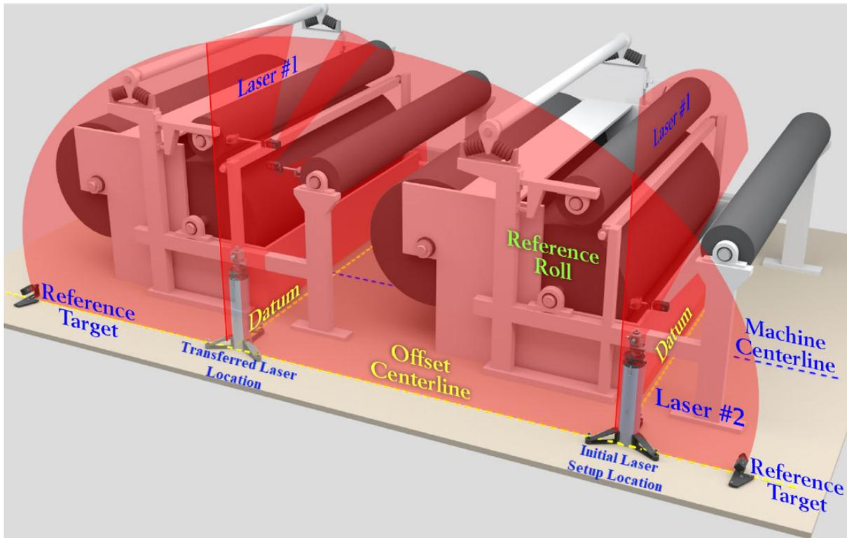
We recommend using a reference roll as the datum for the L-742 setup because when using our Laser Transfer Method, the squareness error between the laser planes is eliminated. And in fact, our Laser Transfer Method can align rolls for as long as a machine is, so even a machine that is 1000 feet (305 m) can easily be aligned with the L-742 without a loss of accuracy!
