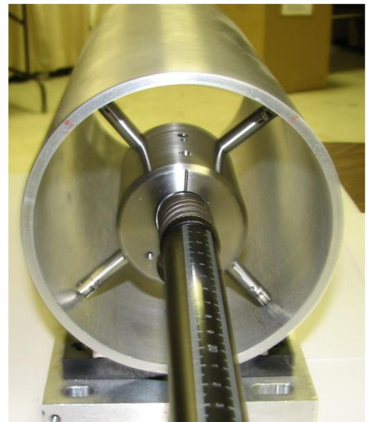
A-516 Self-Centering 2-Axis Bore Target
