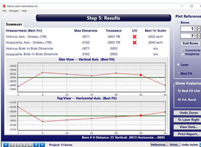
Bore9 – Step 5: Results – Straightness Plot using the Best Fit line as a reference.
