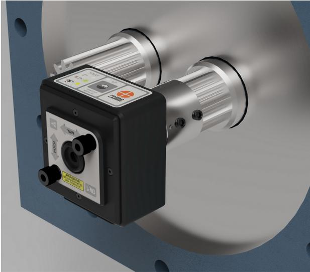
Using components from several different systems, Hamar Laser has developed a package to align twin-barrel extruders as quickly and accurately as possible. Our L-703 Bore & Spindle Laser and A-510 2-Axis Self-Centering Bore Target create a powerful package to align twin-barrel extruders up to 70% faster than conventional or optical borescope methods. With an accuracy of  $\pm 0.0002$  in. (0.005 mm) and our optional alignment software, the L-700 is the perfect extruder alignment tool.
