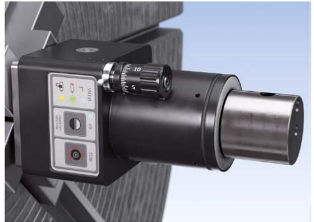
Figure 2 – L-702SP Spindle Laser and Scan Plane
