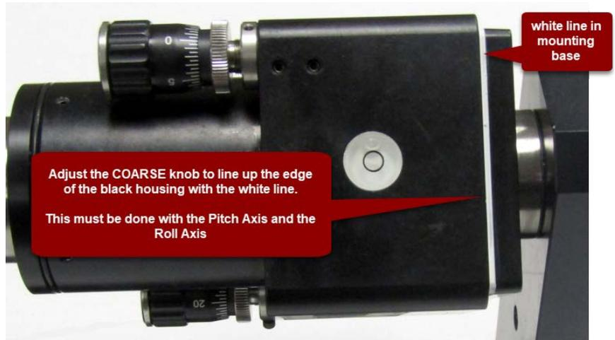
**Figure 11**—Returning the L-702 Pitch/Roll Adjustments to the middle of their range
