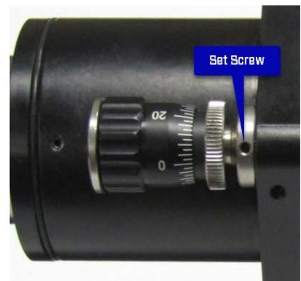
Figure 4– Differential Micrometer
