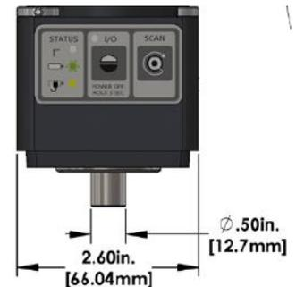
Figure 8—L-702 Mounting Stud
