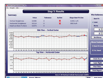
Bore9 – Step 4 Results – Shows a graph of the vertical and horizontal barrel straightness.
