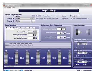
Bore9 – Setup Screen – Enter number of points, distance between points and alignment tolerance for the alignment results.
