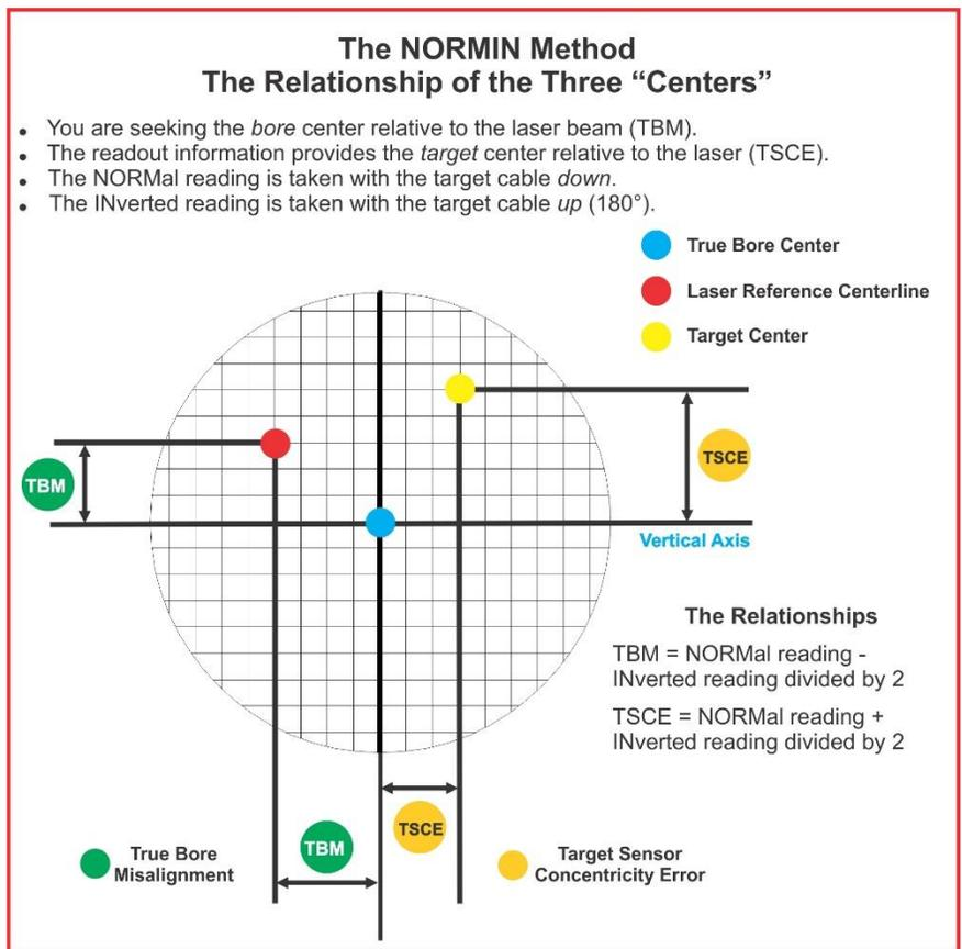
Figure 22 -- Three centers of bore alignment
