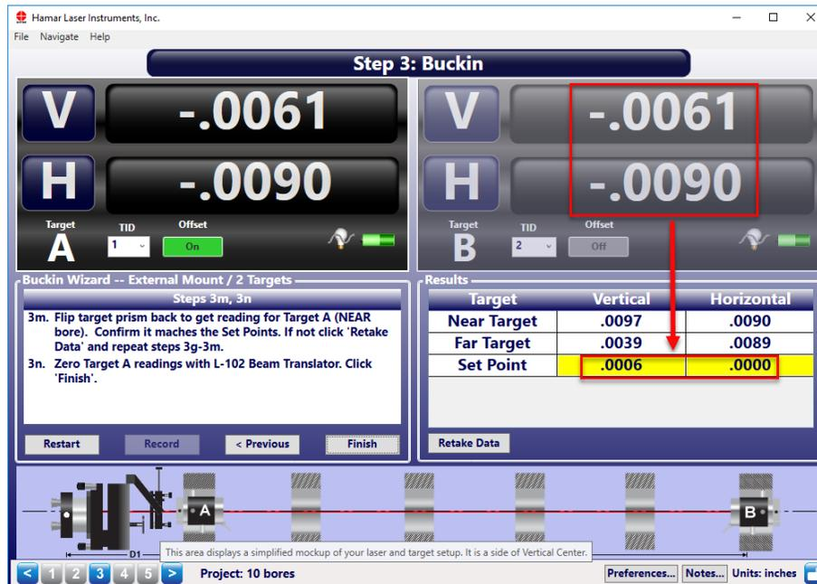
15. Flip the prism on the T-218 Target back into the laser beam and note the reading. The readings should match the **Set Points**. If not, they will be close. Repeat Steps 11-14 to fine tune the setup to get it closer to zero.
