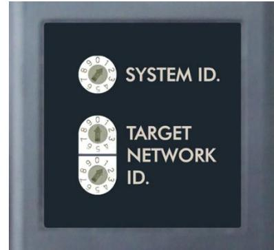
Figure 29 – Unitarget ID Switch set to 1
