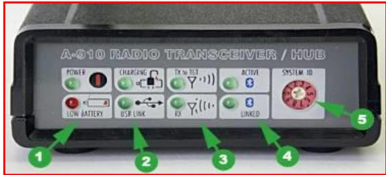
Figure 25 – The A-910 Radio Transceiver/Hub FRONT PANEL
