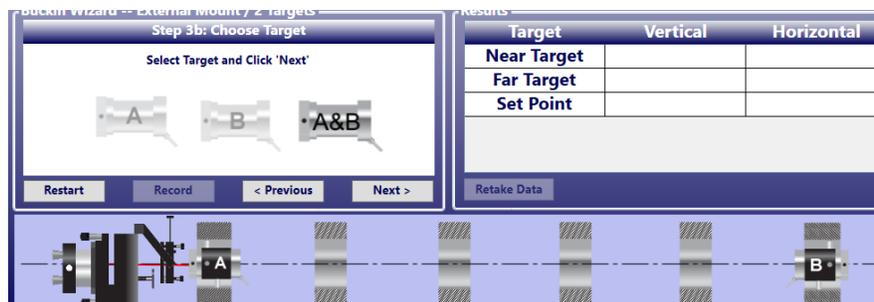
10. Enter the distance from the laser pivot to the Near Target and the distance from the Near Target to the Far Target (see graphic at the bottom screen to see how to measure the dimensions – shown here). Click **Next**.
