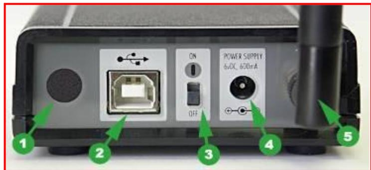
Figure 26 – The A-910 Radio Transceiver/Hub REAR PANEL
