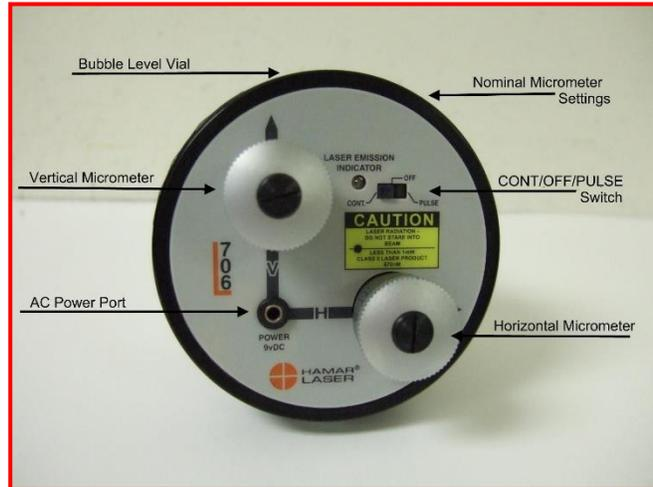
1. Rotate the laser to the INverted position (Vertical Arrow pointed at 6:00) until the bubble is centered in the level vial window.
